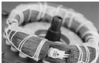
Fig. 50 Thermal switch incorporated in windings
